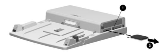
Figure 6-7. Removing a PC Card
